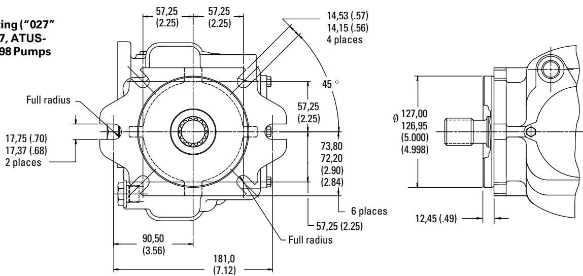
**Cover ("031" Option) for Thru-drive SAE "A" Rear Mounting Flange**
