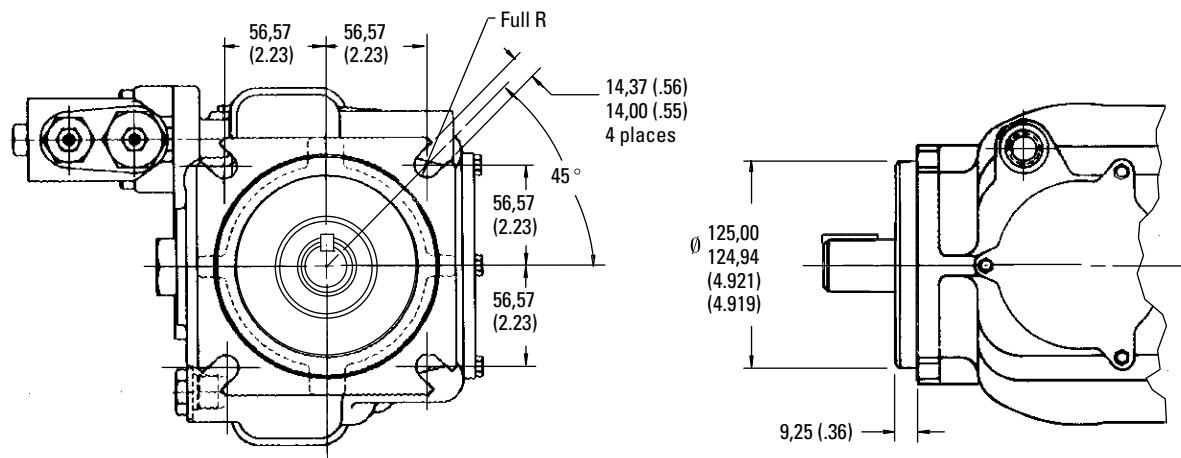
**SAE 2-bolt/4-bolt Mounting ("027" Option) for ATUSP-VH057, ATUS-PVH074 and ATUS-PVH098 Pumps**
