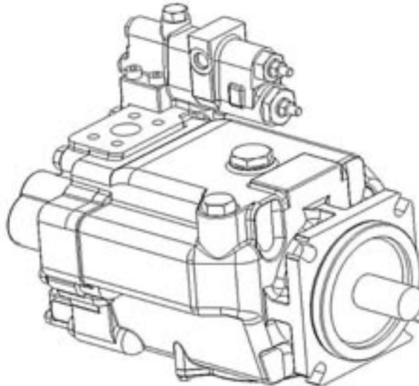
ATUS PVH high flow, high performance pumps are a family of variable displacement, inline piston units that incorporate the proven design, quality manufacturing techniques and operating features of other ATUS piston pumps, but in a smaller, lighter package.
