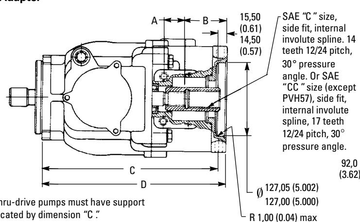
Thru-drive pumps must have support located by dimension "C".
