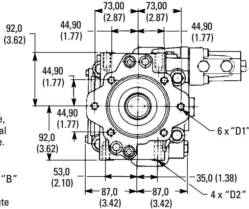
SAE "B" rear mounting. Mounting pad is machined to accept AS568-155 O-ring. Mounting pad is connected to pump case and must be sealed.
