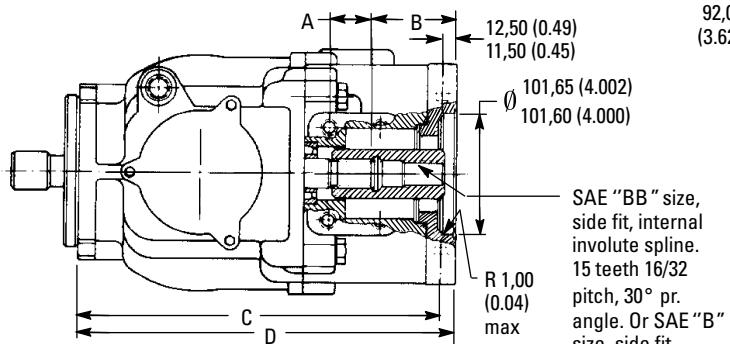
Thru-drive pumps must have support located by dimension "C".
